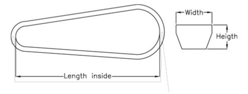
$\begin{array}{ll} \text{Datum Llength} = 3990 \\ \text{Height} & = 10 \\ \text{Length inside} & = 3950 \\ \text{Width} & = 17 \end{array}$
